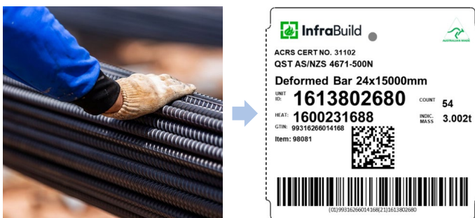
Figure 4. InfraBuild steel bundle data embedded barcode example
